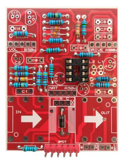
First of all place the IC sockets (without the ICs). Pay attention to the orientation! The small notch in the socket should be oriented as indicated in the PCB.
